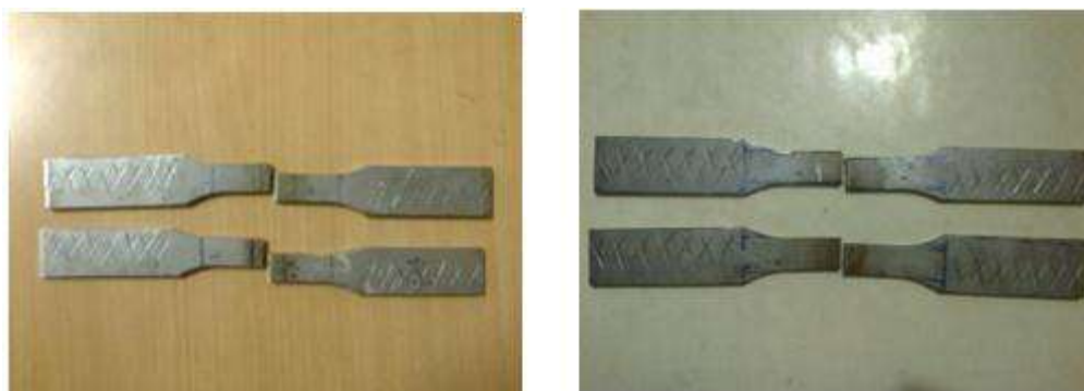
Figure 2: Illustrate the TIG and MIG Testing specimen after tensile test
